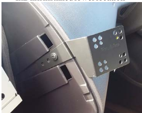
InDash installed upper location
